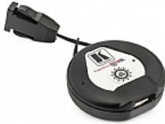
Corona Tag is an innovative device designed to monitor social distancing in the workplace, school, or public venues. It eliminates the need for a wide shutdown in case of infection. Based on HSL technology, Bluetooth signals measure the distance and exposure time between tags without revealing or saving personal information. The device is fully independent, does not rely on cell phones or other connections, and does not require charging.
