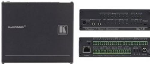
The SL-12 is a master room controller that can operate over Ethernet (LAN) with control ports that include: one bidirectional RS-485, four RS-232, four IR, four GPI/O, and eight relay. It controls devices such as scalers, video displays, audio amplifiers, DVD players, sensors, screens, shades, door locks, and lights. Multiple Kramer Ethernet gateways can be used to add remote I/O ports.
