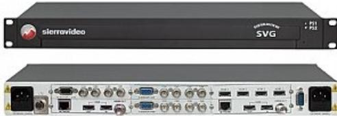
The SierraView SVG MultiViewer uses a modular architecture, allowing customizing of inputs in groups of four for up to 20 inputs with an additional HDMI input on each output module. The three input modules consist of the CV/SD module (auto-sensing CVBS & SD/SDI), the 3G HD-SDI module (auto-sensing SD-HD/SDI), and an HDMI module (with EDID). The output module consists of an HD-SDI output with a cloned HDMI output (to 1920x1080p).
