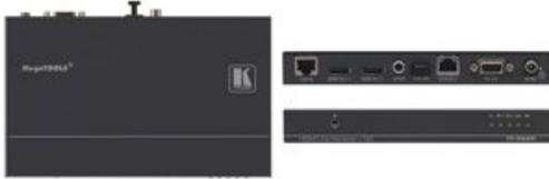
TP-582R is a high-performance, extended-reach HDBaseT receiver for 2 mirrored 1080p60Hz HDMI, Ethernet, RS-232 and IR signals over twisted pair. The TP-582R converts the transmitted HDBaseT signal to all output signals, and de-embeds the audio to S/PDIF and TOSLINK® audio outputs. It extends video signals to up to 130m (430ft) over CAT copper cables at up to 1080p@60Hz 36bpp video resolution
