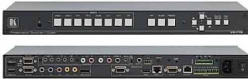
The VP-770 is a high-performance presentation switcher and scaler for composite video, component video, DisplayPort, computer graphics video, and HDMI signals. It scales the video, embeds the audio and outputs the signal to HDMI, computer graphics and DGKat twisted pair, together with digital audio, unbalanced stereo and a 10-watt amplified balanced stereo speaker output
